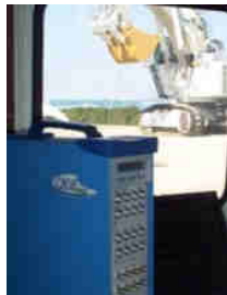
Sound power test on a mine excavator
