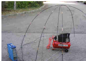
Sound power test on a air compressor
