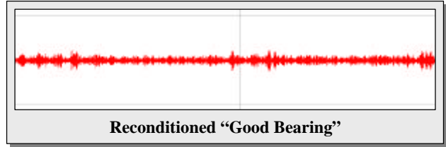
Figure 3 Sample Bearing Time Based Acoustic Signature
